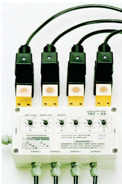
The TEC-55 is supplied complete with the controller, 4 solenoid valves, 2 meter (5' off) cables and DIN connectors.
